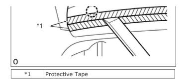
Insert a moulding remover between the outer mirror cover and outer mirror body as shown in the illustration and detach the claw.
