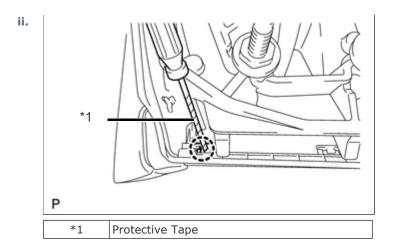
Using a screwdriver, detach the claw.
