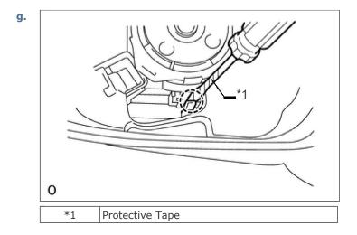
Using a screwdriver, detach the claw.
