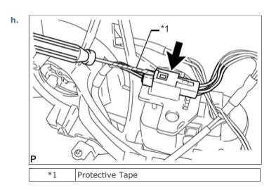
Using a screwdriver, disconnect the connector.
