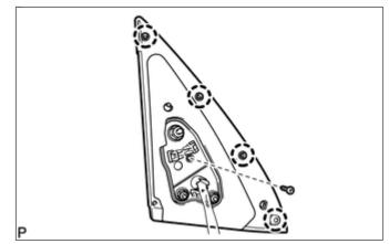
Remove the screw, detach the 4 claws and remove the rubber base.
