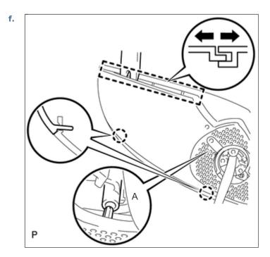
Using a moulding remover, open the mirror body as shown in the illustration.
