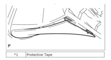
Using a screwdriver, detach the claw to create a space between the lower mirror cover and mirror body as shown in the illustration.
