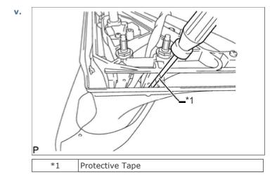
Insert a screwdriver as shown in the illustration.
