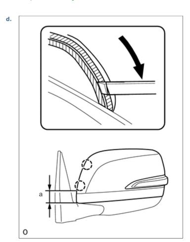
Slide the moulding remover downwards as shown in the illustration to detach the 2 claws.
