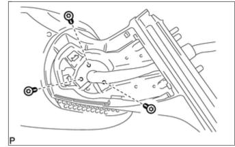
Using a T25 "TORX" socket wrench, remove the 3 screws.
