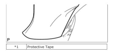
Detach the claw to create a space between the lower mirror cover and mirror body as shown in the illustration. **HINT:**
