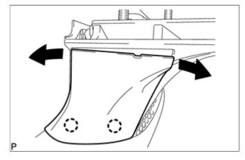
While moving the lower mirror cover back and forth in the directions of the arrows in the illustration, detach the 3 claws and remove the lower mirror cover.
