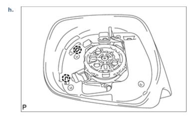
Detach the 2 claws and remove the outer mirror cover.
