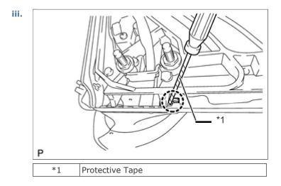
Using a screwdriver, detach the claw.
