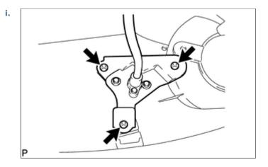
Remove the 3 screws and side television camera.
