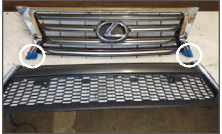
Trim back the ends (circled) to allow bracket and bumper clearance.
