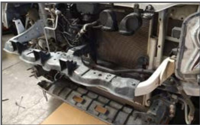
Unbolt the plastic on the center frame section
