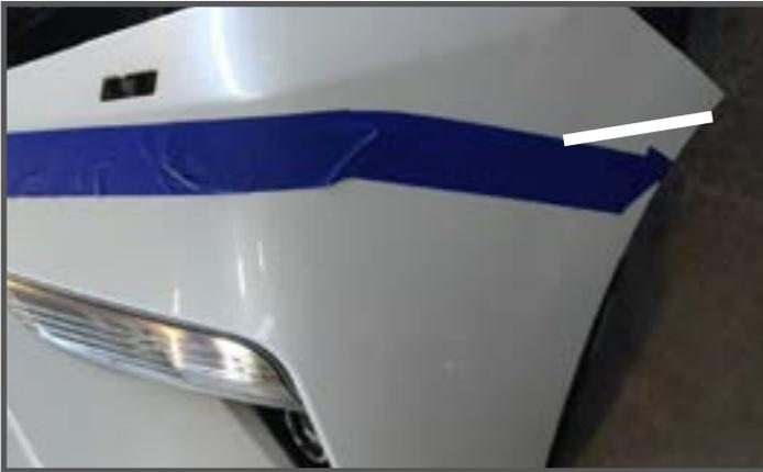
Once cut, notch out the area below the corners to allow clearance for fitting the bumper.
