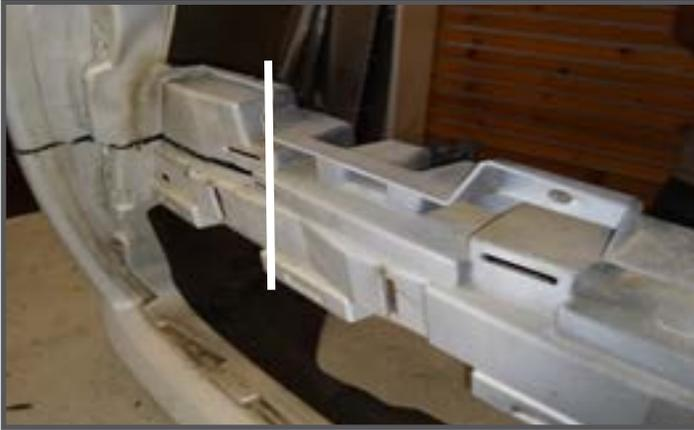
Cut the inside section of the bumper out on both ends.
