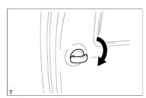
11. REMOVE NO. 1 TONNEAU COVER HOLDER CAP (w/o Tonneau Cover)
