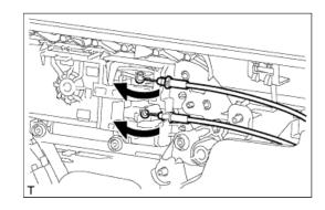
**f.** Disconnect the front door lock remote control cable assembly and front door inside locking cable assembly.
