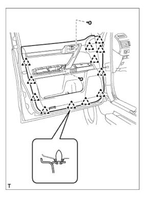
**c.** Pull out the front door trim board sub-assembly in the direction indicated by the arrow in the illustration.
