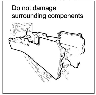
a) Install the front of the console box with rear section lifted as shown.
