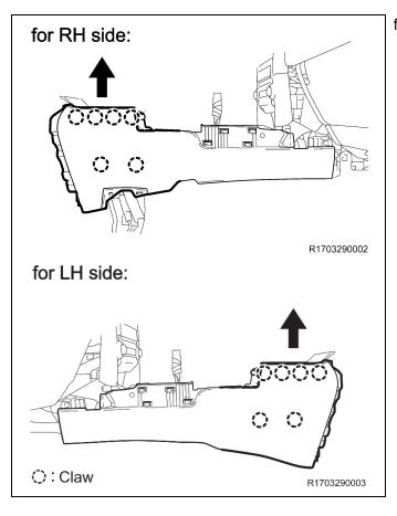
f) Disengage the 6 claws on each side of the console as shown.
