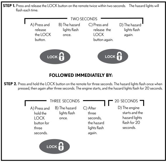
**NOTE:** Vehicles started with the Remote Engine Starter can idle for a total of 20 minutes, however automatic engine shutdown occurs after 10 minutes of run-time. You can always restart the Vehicle after this initial shutdown. Once the total run-time exceeds 20 minutes the vehicle must be manually started inorder to reset the Remot Engine Starter.
