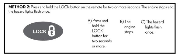
**NOTE:** All doors will remain locked after the engine is shut off.
