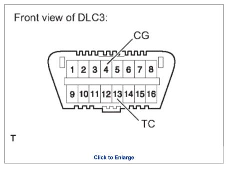
Using SST, connect terminals 13 (TC) and 4 (CG) of the DLC3.
