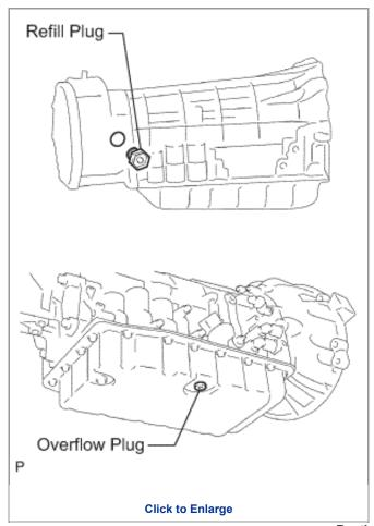
Fill the transmission through the refill hole until fluid begins to trickle to trickle
