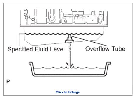
Check that the fluid comes out of the overflow tube.
