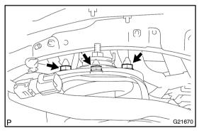
(b) Install the 3 nuts on the upper side of the front shock absorber with coil spring.
