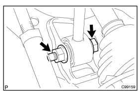
(c) Temporarily tighten the bolt, the nut and the washer as shown in the illustration.
