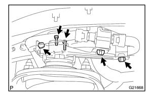
(e) Install the absorber control actuator with the 2 bolts.
