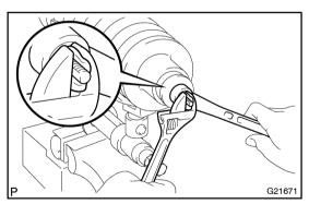
(b) Hold the shock absorber rod, and remove the nut. **NOTICE:**
