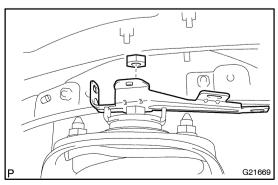
(c) Remove a nut and the bracket.
