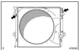
Remove the 2 bolts, and separate the fan shroud. (e) HINT:
