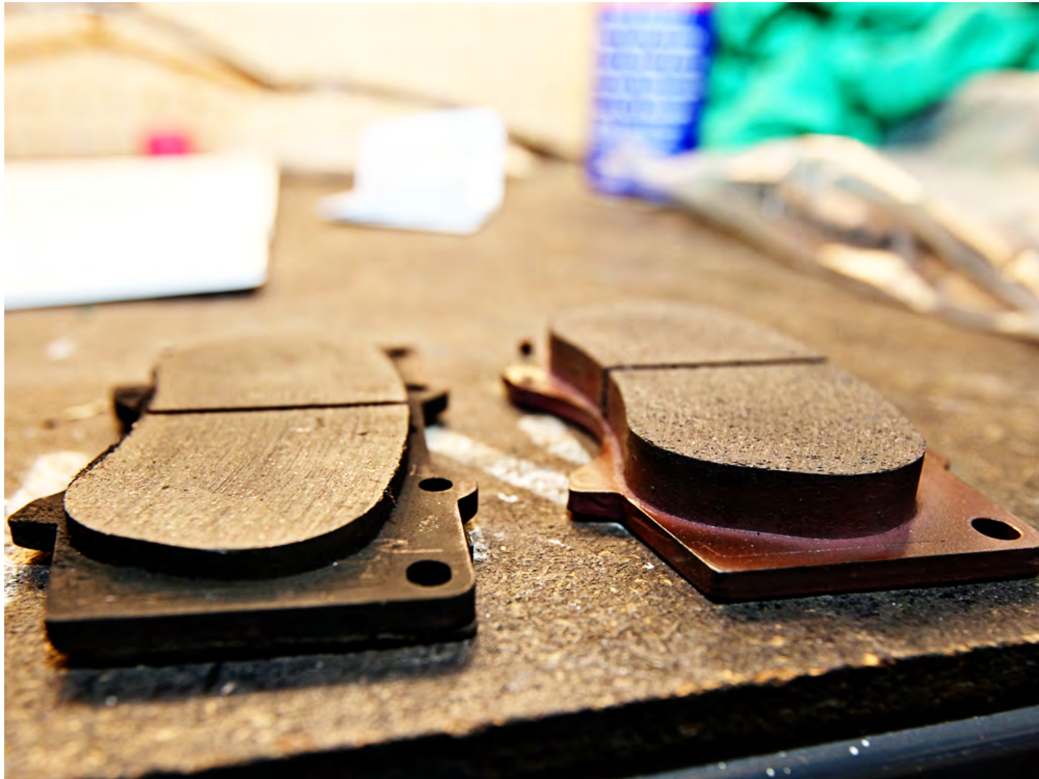
Old Pad and New Pad.
