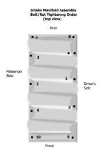
27. After you've bolted the intake manifold assembly into place, finish reassembly by reversing the steps. When bolting the Throttle Body back onto the intake manifold, use your torque wrench to tighten the four nuts and bolts to **13 foot-pounds**.
