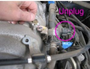
8. Unplug all fuel injectors. There are four, blue fuel injectors with connectors nestled below the fuel rails on either side of the intake manifold assembly. The fuel rails are pipes with a fine, waffle-print pattern on them. The upper part of the blue fuel injectors plug into the fuel rails, and the lower part of the injectors plug into the intake manifold.
