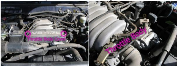
4. Remove and label vacuum lines, cable bundle support, and hose bracket from air intake hose. There are four rubber hoses and a cable bundle connected to the rectangular box on the air intake hose, and a hose mount bracket on the front of the air intake hose. For sanity's sake, we placed
