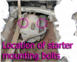
19. Once you've unbolted the starter, rotate starter counterclockwise a little bit and unplug the exciter wire and remove 12mm nut holding battery wire to starter. The nut is located under a cap.
