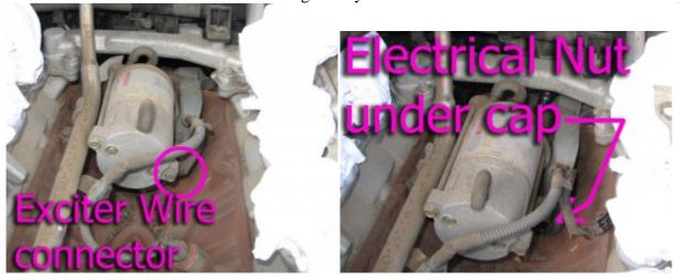
20. Here's a photo of the new starter in place, showing the electrical connector nut and the socket for the exciter wire.
