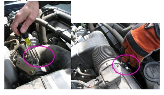
6. Unplug the large connector from the air intake box.
