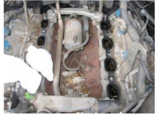
17. Remove 12mm bolt connecting the wire harness to the starter. This bolt is reached from behind the engine. The bolt is hard to get to, as you have to reach your socket wrench between the firewall and the head block. You need to do this by touch, and there is hardly any room to operate the wrench. Again, your magnetic grabber is helpful here to retrieve the bolt as you
