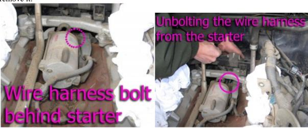
18. Remove the two 14mm bolts holding the starter to the block. Again, you reach these bolts from the back. These are even harder to get to than the bolt in step 17. If you need guidance, take a look at the bolt holes on your new starter to guide you. You'll need to experiment with extensions and deep vs. regular sockets to get the best results. At least the heads on these bolts are extra long, which makes them easier to get to.
