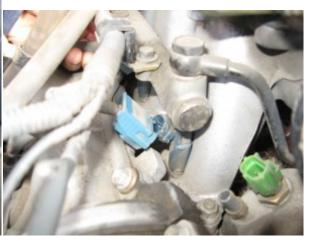
9. Unbolt the throttle cable from the front bracket. There are two nuts sandwiching the fingers of the bracket Just loosen the front nut.
