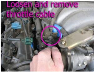
10. Unbolt the Throttle Body. Pull it away from the intake manifold and move it to the side. You don't have to drain coolant or remove any hoses. Pull the gasket away from the intake manifold. If you're planning on reusing it, set it aside where you won't damage it.
