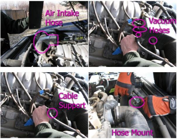
5. Remove air intake hose by loosening the hose clamps at the air intake and the throttle body and wiggling the hose free.
