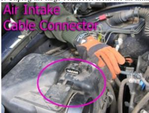
7. Intake Manifold Assembly: Remove and label vacuum lines. Unbolt throttle cable bracket and assorted cable mount brackets. Unplug cable connector from the small black box on the driver's side of the intake manifold. Make sure that you don't mistakenly unbolt the fuel rail connectors.
