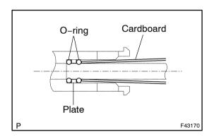
(2) Insert the tube on which 2 O-rings and a plate are installed into the housing, and then push it in lightly with rolled up cardboard.
