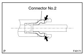
(3) Push the connector No.2 into the housing to the position where a clicking sound is heard.
