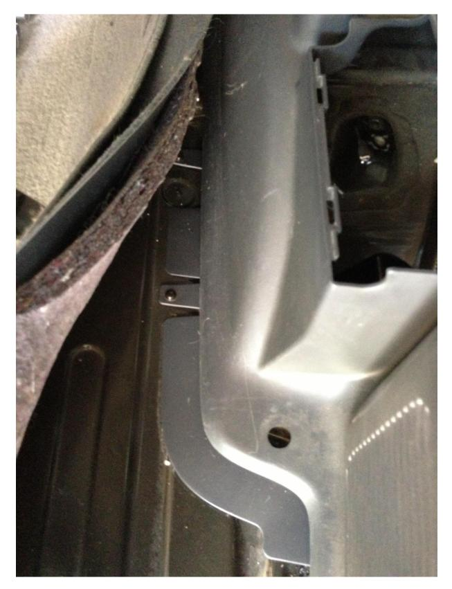
Pull back the carpet to expose the screws holding the rear side panel in place and remove the screws.
