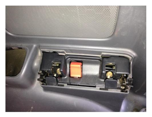
Remove the cover from the third row seat attachment, if applicable and pry back the covers on each side of the orange release button and remove the bolts. The assembly will lift out.
