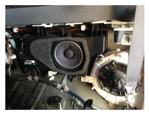
Remove the bolt and metal plate holding the rear air in place to allow the sub to be removed.
