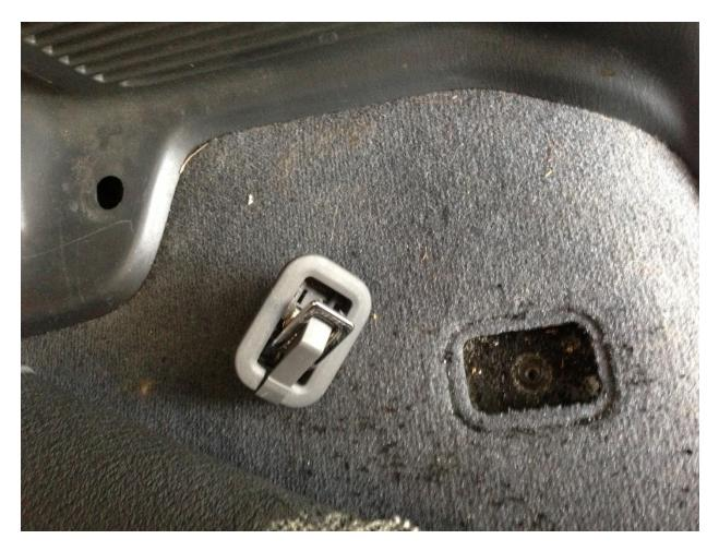
There's also a cover over the rear tie downs that simply preys up exposing the bolt. Both front and rear ones will have to be removed.
