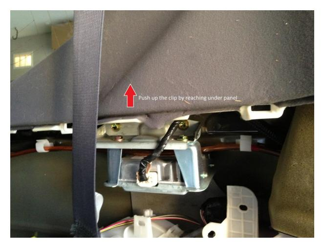
The speaker box assembly can now be removed.
