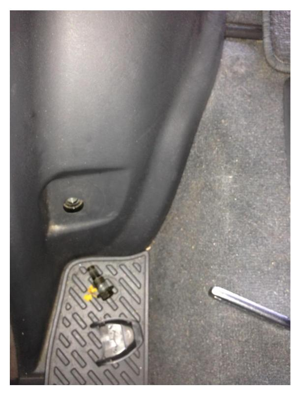
The rear passenger seatbelt, step and trim can be removed in the same fashion as the rear. The panel can now be removed, exposing the sub. There is a pug attached to the 110 outlet, so use caution not to break it when detaching.
