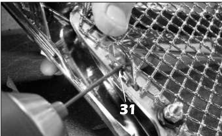
31. Use a 7/64" drill bit to drill through the factory mounting tabs once the mesh and surround have been pressed firmly against the factory chrome frame.
