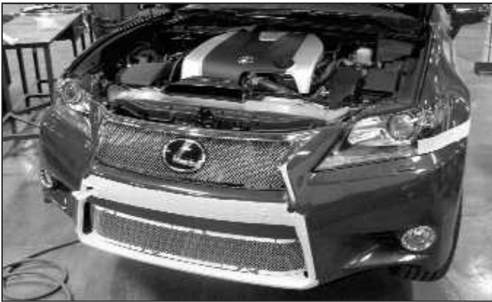
49. With the help of an assistant, realign the bumper cover back onto the vehicle. Reverse the removal procedure to reinstall the bumper cover.
