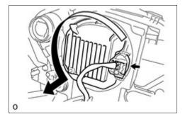
(b) Turn the headlight light control ECU sub-assembly LH in the direction indicated by the arrow in the illustration and separate the headlight light control ECU sub-assembly LH from the headlight unit.
