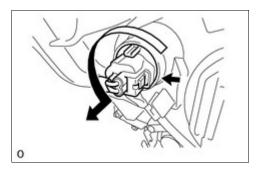
(b) Turn the front turn signal light socket in the direction indicated by the arrow in the illustration and remove the front turn signal light socket.
