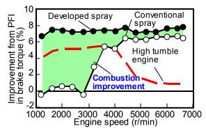
Fig. 13 Improvement in torque from a PFI engine
