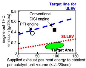
Fig. 18 Direction and strategy for reduction of the exhaust emissions
