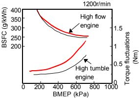
Fig. 4 Comparison of fuel consumption and torque fluctuations between the high flow engine and the high tumble engine for part loads at 1200r/min
