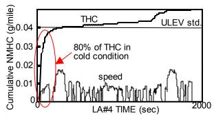
Fig. 17 Transition of HC emissions for FTP mode
