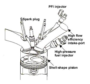
Fig. 5 A perspective view of the combustion chamber geometry of D-4S system
