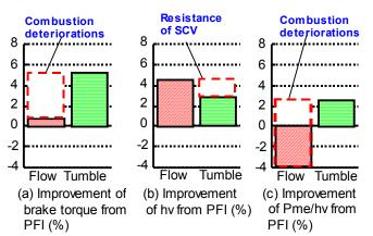
Fig. 2 Improvement of brake torque from a PFI engine at 2800r/min
