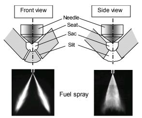
Fig. 6 Dual-fan-shaped spray shape
