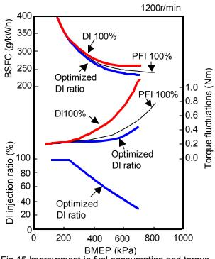
Fig.15 Improvement in fuel consumption and torque fluctuations of D-4S system
