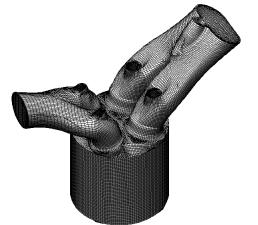
Fig. 8 CFD model of test engine
