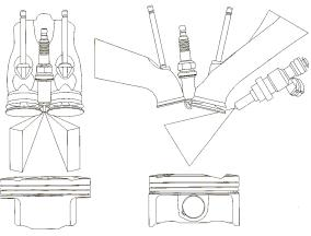
Front view Side view Fig. 7 Schematic view of in-cylinder pattern of the newly developed spray
