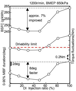
Fig.14 Improvement of combustion with simultaneous injection
