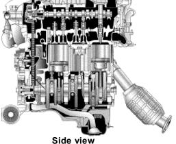
Fig. 21 Section view of the 2GR-FSE
