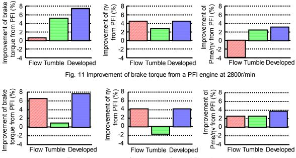
Fig. 12 Improvement of brake torque from a PFI engine at 6400r/min
