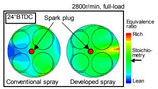
Fig. 10 Comparison of the mixture formation of the developed spray at the cross section of the spark plug
