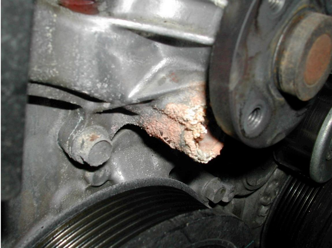
Next I removed the injector drive. 2 10mm nuts and 1 10mm bolt (underneath – don't miss this). I then just put it out of the way – no need to completely remove electrical lines.
