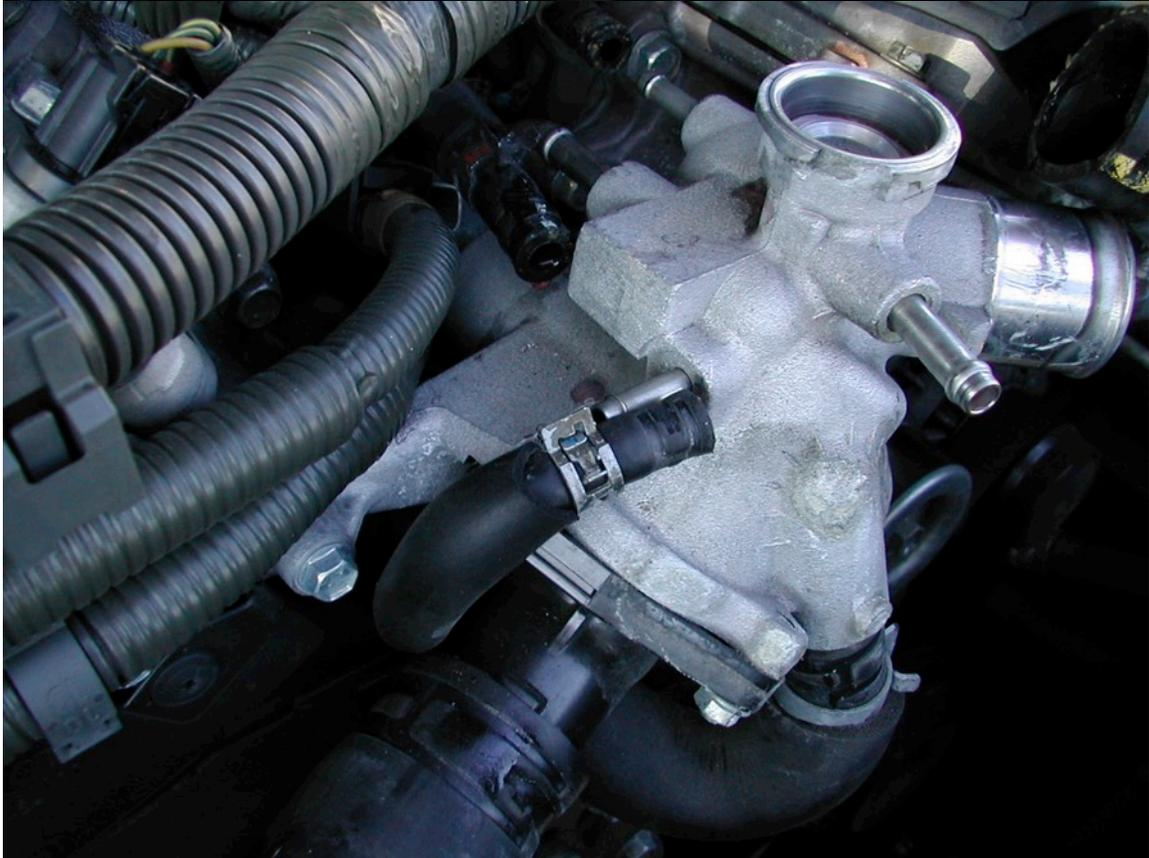
I went ahead and loosened water pump pulley. 4 bolts, all 12mm. The tension on the belt allows you to break loose so you do not need a special tool.
