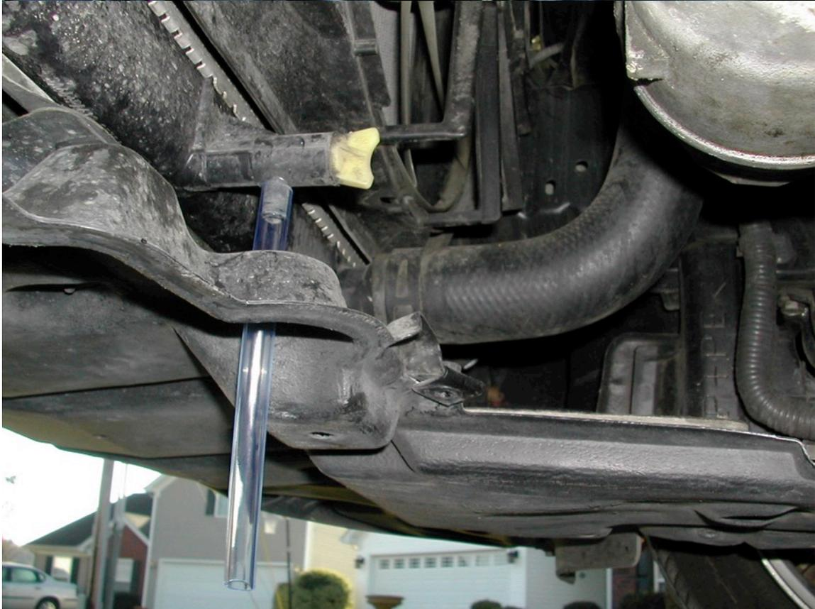
I also removed reservoir, drained and cleaned. Easy – two 10mm bolts.
