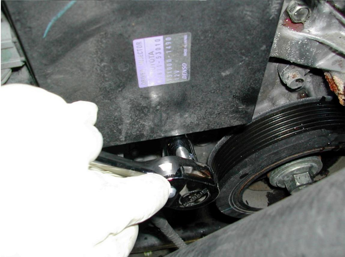
Next I removed both the idler pulley (already removed in 1<sup>st</sup> pic. I replaced this) and the tensioner pulley. The tensioner blocks 1 of the 16 bolts that holds the water pump assembly.
