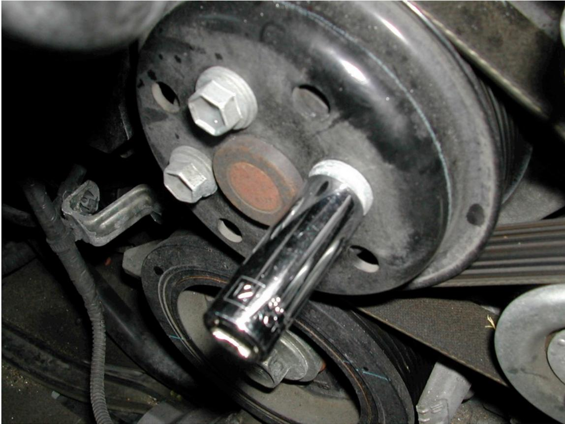
Next I removed the belt. Use 14mm wrench on tensioner pulley, pulling toward water pump pulley – this allows you to free tension and belt. Overall belt didn't look too bad.
