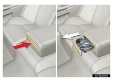
To open, press in and release the rear cup holder on the armrest.
