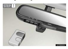
Point the remote control for the device 1 to 3 in. (25 to 75 mm) from the HomeLink® control buttons.
