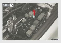
Remove the fuse with the pull-out tool.
