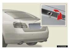
Turn the mechanical key clockwise to open.
