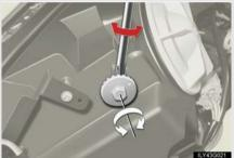
Using a Phillips-head screwdriver, turn adjustment bolt A so that the bubble is within the 2 center lines.
