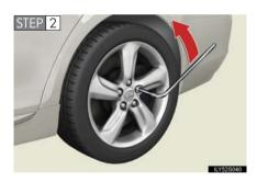
Slightly loosen the wheel nuts (one turn).
