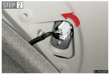
Partly remove the trunk panel cover and turn the bulb bases counterclockwise.
