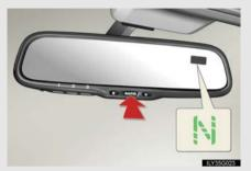
To turn the compass on or off, press "AUTO" for 3 seconds.
