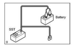
(2) Press the SST activation switch and check that the LED of SST activation switch illuminates.
