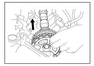
**Repair** 36. Install the No. 3 camshaft.
