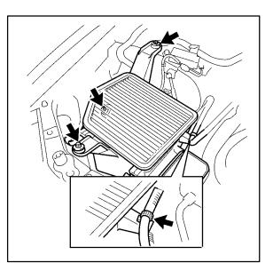
Repair 60. Install the air cleaner cap with air Procedure (Continued)
