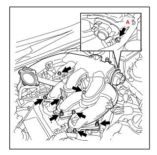
D. Install the surge tank stay to the intake air surge tank.
