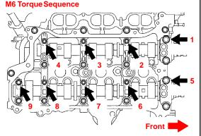
E. Tighten the 9 M8 bolts in the sequence shown in the illustration.
