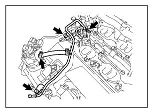
Repair 17. Disconnect fuel pipe No. 2.
