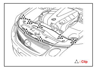
3. Remove the engine compartment side cover RH by removing 2 clips.
