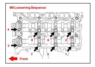
**Repair** 31. Remove the No. 2 camshaft.
