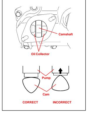
C. Apply a coat of engine oil to the pump activation cam and pump lifter part.
