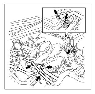
D. Disconnect the ventilation hose from the intake air surge tank.
