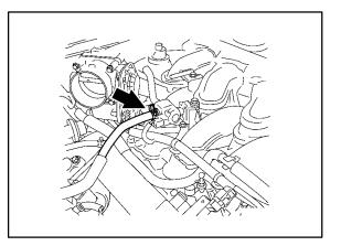
**Repair** 13. Disconnect the fuel main tube.
