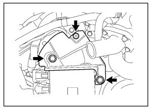
46. Install the cylinder head cover RH.
