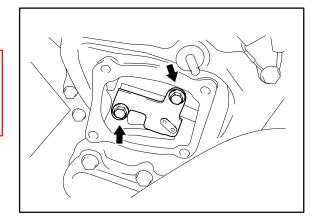
**Repair** 29. Remove the timing chain.
