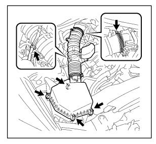
10. Remove the air cleaner case sub-assembly by removing 3 bolts, clamp, and the case.
