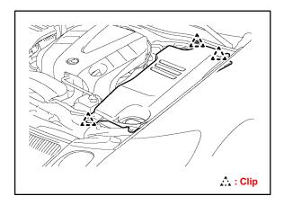
71. Install the engine compartment side cover RH with the 2 clips.
