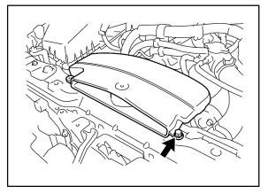
Disconnect the No. 2 ventilation hose from the cylinder head.
