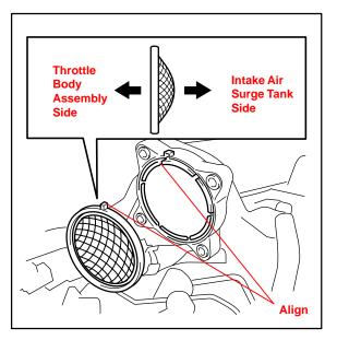
B. Install the throttle body with the 4 bolts.
