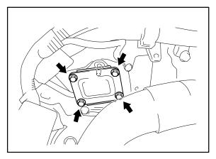
44. Install the injector driver with the bolt and 2 nuts. Torque: 10 N•m (102 kgf•cm, 7 ft•lbf)
