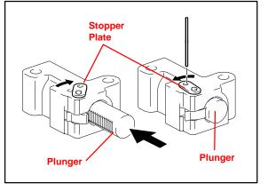
C. Install the No. 1 chain tensioner assembly with the 2 bolts.
