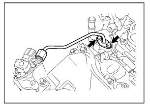
B. Using a 19-mm union nut wrench, connect the fuel pipe.
