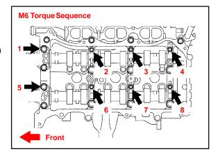
E. Tighten the 8 M8 bolts in the sequence shown in the illustration.
