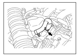
Repair<br/>Procedure<br/>(Continued)62. Install the No. 1 air cleaner inlet with<br/>the bolt and clip.
