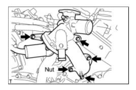
(b) Remove the 4 bolts, nut and water inlet.
