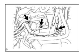
(a) Remove the 3 nuts and engine harness cover (LH bank side).
