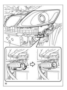
(a) Disconnect the connector as shown in the illustration.
