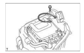
(a) Remove the screws and headlight protector.
