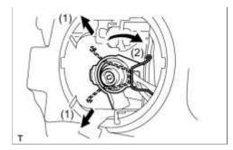
(b) Release the set spring lock as shown in the illustration and remove the bulb.
