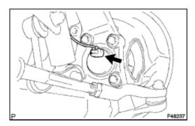
(a) Disconnect the speed sensor connector from the speed sensor front.
