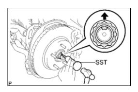
(a) Using SST and a hammer, release the staked part of the front axle hub nut.
