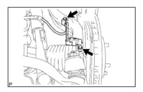
(a) Remove the 2 bolts, and separate the speed sensor from the steering knuckle.
