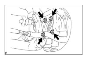
(a) Using a plastic hammer, separate the front drive shaft assembly from the front axle hub.
