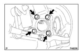
(a) Remove the 4 bolts, front axle hub sub-assembly and front disc brake dust cover.
