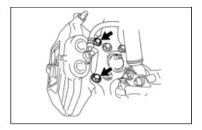
(a) Remove the 2 bolts, and disconnect the brake caliper assembly.
