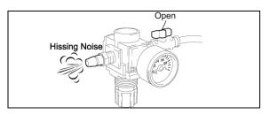
c) Open the valve to release the residual pressure.
