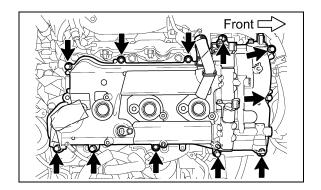
f) Apply adhesive 1324 to the threads and install the valve cover bolts. Do not torque yet.
