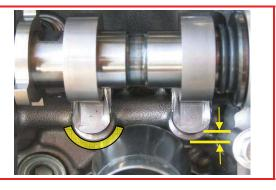
After installing the camshafts, confirm all rocker arms are correctly installed - Check for a consistent "U" shape distance.
