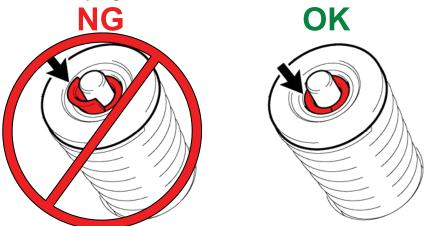
If the keepers are not properly installed The valves will drop in to the cylinder.
