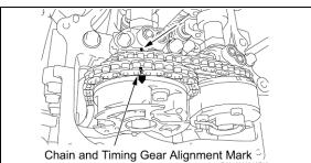
Align the chain so that it matches up with the timing marks and paint marks made before disassembly.
