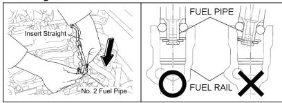
NOTE: Pushing at an angle can cause scratches and nicks which will potentially cause fuel leaks.
