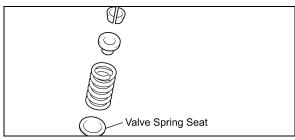
d) Although it should stay in place, confirm the valve spring seat is still seated on the cylinder head after spring removal.
