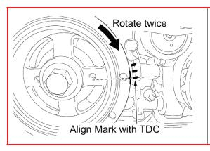
g) Rotate the engine 720° and stop at the TDC mark.
