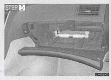
Push the tabs and remove the filter case.
