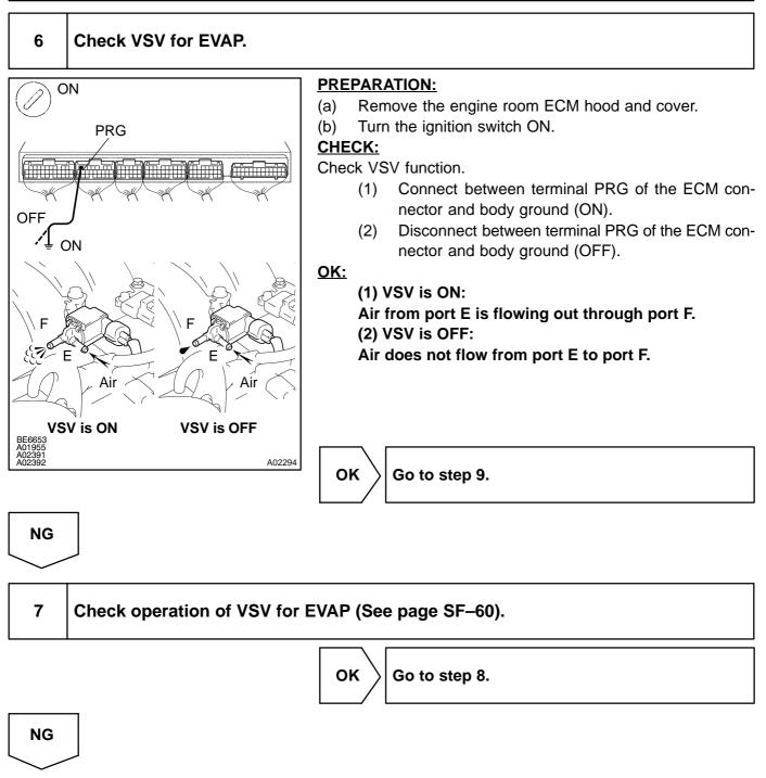
Replace VSV and charcoal canister, and then clean vacuum hoses between throttle body and VSV for EVAP, and VSV for EVAP and charcoal canister.
