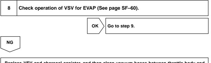
Replace VSV and charcoal canister, and then clean vacuum hoses between throttle body and VSV for EVAP, and VSV for EVAP and charcoal canister.
