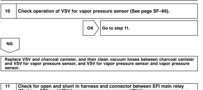
(Marking: EFI) and VSV for vapor pressure sensor, VSV for vapor pressure sensor, and ECM (See page IN–31).
