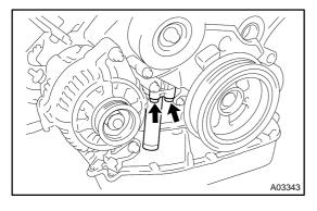
Alternately loosen the 2 bolts, and remove them, the belt tensioner and dust boot.
