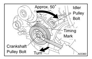
(c) Turn the crankshaft pulley approx. 50° clockwise, and put the timing mark of the crankshaft pulley in line with the centers of the crankshaft pulley bolt and the No.2 timing belt idler pulley bolt.
