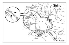
When replacing timing belt tensioner only:
