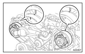
(b) Check that the timing marks of the camshaft timing pulleys and timing belt rear plates aligned.
