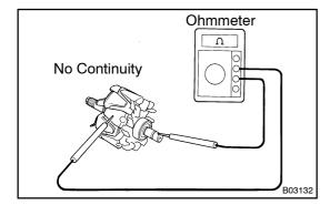
(b) Check the rotor for ground.Using an ohmmeter, check that there is no continuity between the slip ring and rotor.
