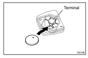
(e) Install a battery (lithium battery) as shown in the illustration.
