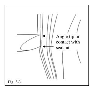
Sealant Issue: To push back sealant; align the adjustment tool to the edge of the door, with the angle edge positioned toward the inside of the door (Fig. 3-3).
