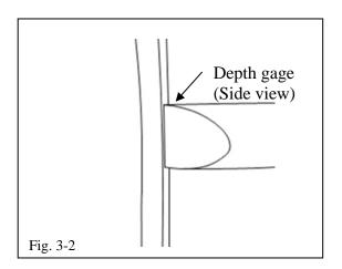
Align the adjustment tool to the edge of the door, with the angle edge positioned toward the inside of the door (Fig. 3-2).
