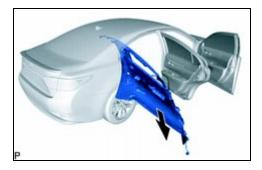
(m) Remove the 3 clips from the vehicle body as shown in the illustration.
