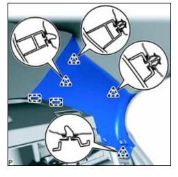
(a) Disengage the 4 clips.
