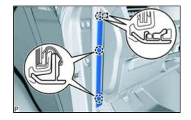
(b) Disengage the guide and remove the front door opening trim cover LH.
