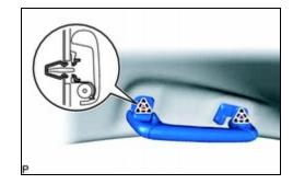
(c) Remove the 2 clips from the vehicle body.
