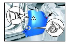
(b) Disengage the claw and clip, and remove the cowl side trim board LH.
