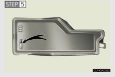
Remove the fuse with the pullout tool. 4
