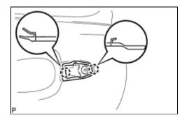
(a) Disengage the 2 claws and remove the rear door rear outside handle pad.
