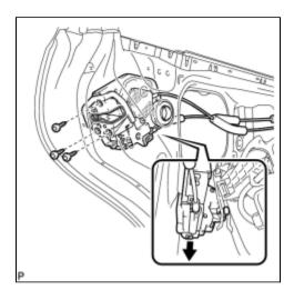
(a) Using a "TORX" socket wrench (T30), remove the 3 screws.
