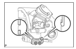
(a) Using a screwdriver, disengage the 3 claws.
