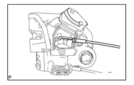
(b) Remove the rear door lock remote control cable assembly.
