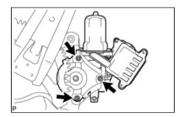
(a) Using a "TORX" driver (T25), remove the 3 screws and the rear power window regulator motor assembly.
