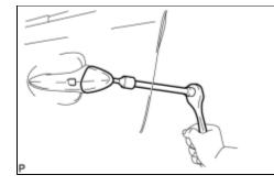
(a) Using a "TORX" socket wrench (T30), loosen the screw.
