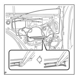
(a) Remove the rear door glass sub-assembly from the rear door window regulator sub-assembly as shown in the illustration.
