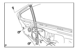
(a) Remove the 2 bolts, the screw, and the rear door window division bar sub-assembly.
