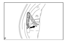
(c) Pull and hold the release plate of the outside handle frame as shown in the illustration.
