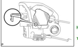
(a) Using a screwdriver, disengage the claw.
