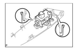
(a) Disengage the 2 claws and remove the rear power window regulator switch assembly.
