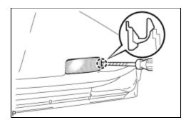
(a) Using a screwdriver with the tip wrapped with protective tape, disengage the claw and remove the courtesy light assembly.
