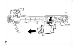
(a) Remove the screw and the door electrical key oscillator.
