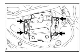
(a) Remove the 4 screws and the rear door inside panel reinforce.
