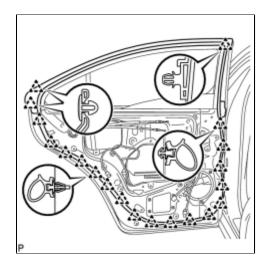
(a) Using a clip remover, disengage the 20 clips and remove the rear door weatherstrip.
