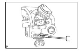
(b) Remove the rear door inside locking cable assembly.
