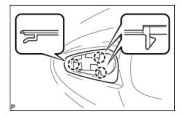
(a) Disengage the 3 claws and remove the rear door front outside handle pad.
