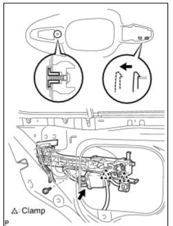
(a) Using a "TORX" socket wrench (T30), loosen the screw.
