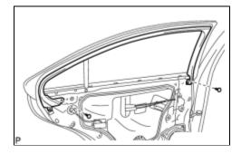
(a) Using a clip remover, remove the 2 clips and rear door frame garnish.
