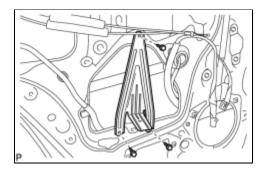
(a) Remove the 3 screws and the rear door trim bracket.
