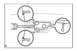
(a) Using a screwdriver with the tip wrapped with protective tape, disengage the 3 claws and remove the rear door inside handle bezel plug.
