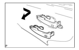
(d) Remove the rear door outside handle assembly as shown in the illustration.
