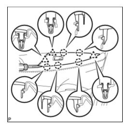
(a) Using a screwdriver with the tip wrapped with protective tape, disengage the 5 claws and 3 clips, and remove the rear door armrest base panel assembly.
