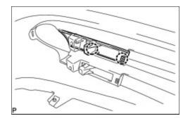
(a) Disengage the 2 claws and radiator grille garnish.
