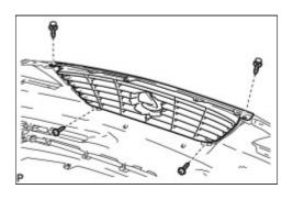
(a) Remove the 2 screws and 2 clips.
