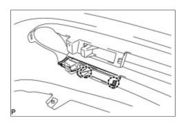
(a) Disengage the 2 claws and No. 2 radiator grille garnish.
