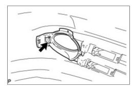
(a) Disengage the claw and remove the fog light bracket LH.
