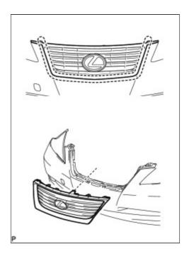
(b) Disengage each claw and remove the radiator grille and radiator grille moulding.
