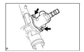
(c) Remove the 2 bolts and the power steering control valve assembly.
