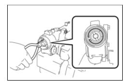
(a) Using needle-nose pliers, remove the cylinder end stopper hole snap ring from the power steering rack housing.
