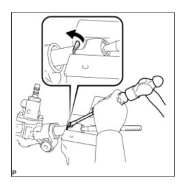
(a) Using a screwdriver and a hammer, unstake the RH and LH claw washers.
