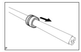
(a) Remove the power steering rack bushing from the power steering rack sub-assembly.
