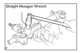
(a) Using a straight hexagon wrench (24 mm (0.94 in.)), remove the rack guide spring cap.
