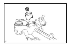
(b) Remove the compression spring and the rack guide sub-assembly.
