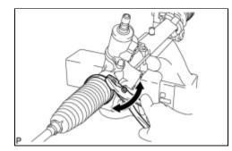
(a) Using pliers, remove the 2 No. 2 steering rack boot clamps as shown in the illustration.
