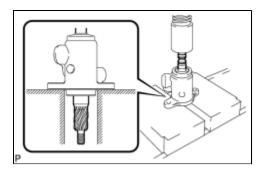
(a) Using a press, remove the power steering control valve sub-assembly.
