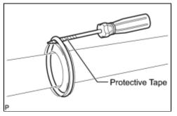
(a) Using a screwdriver, remove the power piston oil seal and the O-ring from the power steering rack.
