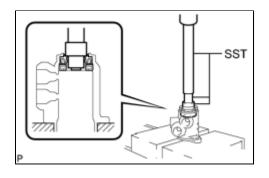
(a) Using SST and a press, press out the power steering control valve upper oil seal and the power steering control valve upper bearing from the control valve housing sub-assembly.
