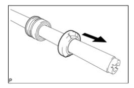
(a) Remove the cylinder end stopper from the power steering rack subassembly.
