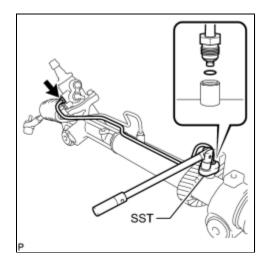
(a) Using SST, remove the steering left turn pressure tube.
