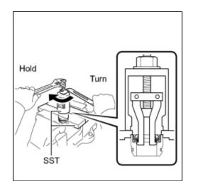
(c) Using SST, remove the rack bushing oil seal from the power steering rack bushing.
