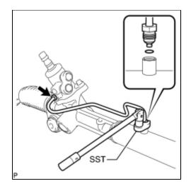
(b) Remove the 2 O-rings from the steering right turn pressure tube.
