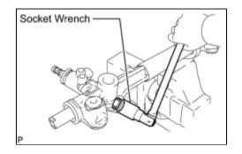
(a) Using a socket wrench (27 mm (1.06 in.)), remove the rack housing cap.
