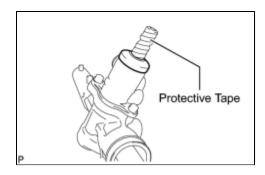
(a) Wrap protective tape around the spline of the control valve in order to prevent damaging the dust cover.
