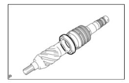
(a) Remove the power steering control valve lower oil seal from the power steering control valve sub-assembly.
