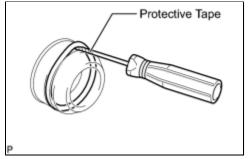
(b) Using a screwdriver, remove the O-ring from the power steering rack bushing.
