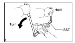
(b) Using SST, hold the control valve shaft and remove the nut.SST: 09616-00011
