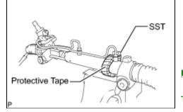
(a) Using SST, secure the power steering link assembly.
