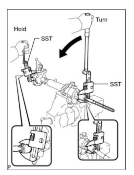
(b) Using SST, remove the steering rack end sub-assembly (RH side) and the claw washer.
