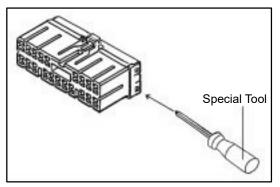
Type B (For 1.8, 1.0 and TLC of Non–Waterproof Type Connector)
