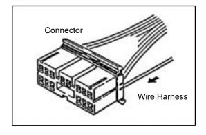
(b) Push the terminal gently into the connector and hold it in this position.
