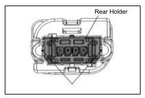
(2) Release Rear holder. Insert Special Tool at the location shown in the figure left.
