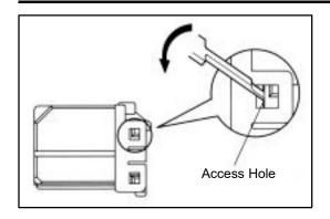
Press the special tool at a 45° angle into the locking lug access hole as shown.
