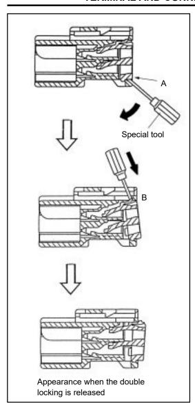
(1) Insert the special tool into the service hole and move it to the direction of the arrow to release the lock on the side A.
