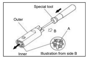
(2) Insert the special tool into the outer shown in the illustration. Then push the area A of the inner and remove the inner from the outer.
