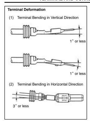
5. Inspect the terminal and the connector for damage.
