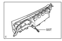
(1) Connect the SST connector to the front passenger side knee airbag assembly.
