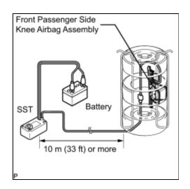
secondary lock of the twin lock. Also, secure some slack for the SST wire harness inside the tire.
