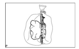
(h) Dispose of the front passenger side knee airbag assembly.
