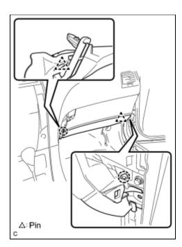
(c) Disengage the 2 claws and 2 pins, and remove the front passenger side knee airbag assembly.
