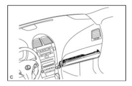
(b) With the front passenger side knee airbag assembly installed on the vehicle, perform a visual check. If there are any defects as mentioned below, replace the front passenger side knee airbag assembly with a new one:
