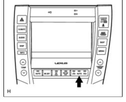
(c) Push the "R/F" switch to perform the actuator check.
