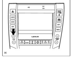
(e) If the steps are difficult to read because they change automatically, push the "UPDr" switch to display the steps one at a time so that they can be read easily. The items are displayed step by step each time the "UPDr" switch is pushed.
