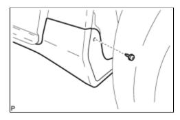
(f) Using a 4 mm hexagon wrench, install the screw.
