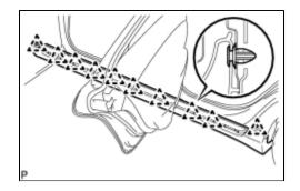
(a) Engage the 10 clips and install the rocker panel moulding sub-assembly.
