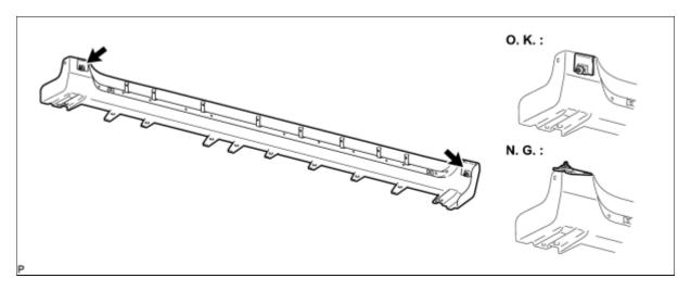
If any of the clip installation portions are not attached securely, replace the double-sided tape by following the procedures below:
