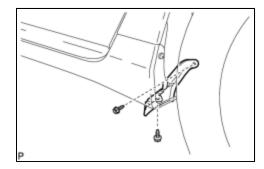
(a) Install the rocker panel moulding protector with the 2 screws.
