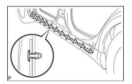
(a) Engage the 12 claws and install the front door weatherstrip.
