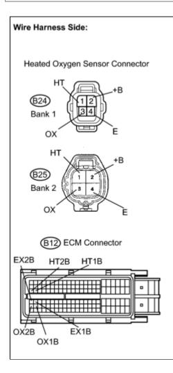
(a) Disconnect the B24 heated oxygen sensor connector (Bank 1 Sensor 2) or B25 heated oxygen sensor connector (Bank 2 Sensor 2).
