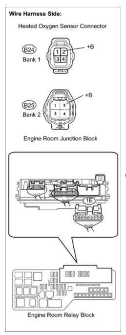
(a) Disconnect the B24 or B25 heated oxygen sensor connector.
