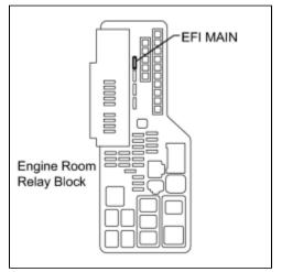
(a) Remove the EFI MAIN fuse from the engine room R/B.
