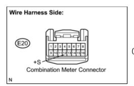
(a) Disconnect the E20 combination meter connector.
