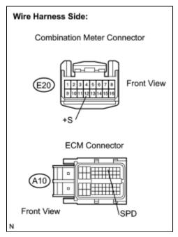
(a) Disconnect the E20 combination meter connector.
