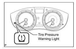
(a) When the tire pressure warning light comes on, immediately check the tire pressure of the tire and adjust it to the specified value. (The tire pressure warning light will come on after blinking for 1 minute if there is an open in the tire pressure warning light circuit.)
