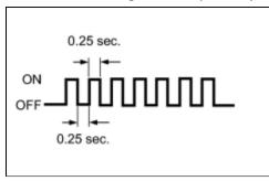
\*5: When determining if there is a short circuit (10 seconds), the light is off. Then it blinks at 0.5 second intervals, and comes on after 1 minute.
