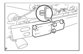
(a) Engage the 4 claws and install the rear bumper arm LH.
