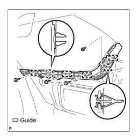
(a) Engage the clip, claw and 4 guides, and install the rear bumper side support LH.
