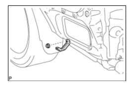
(a) Install the wheel house reinforcement LH with the nut.
