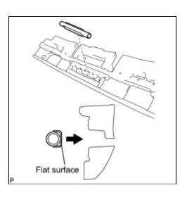
(a) Install the rear bumper bar as shown in the illustration.
