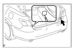
(b) Using a screwdriver, open the 2 rear bumper plates.
