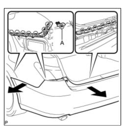
(f) Disengage the 14 claws and disconnect the rear bumper assembly as shown in the illustration.
