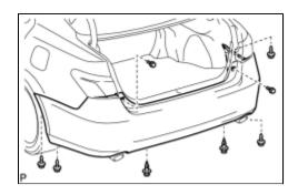
(e) Remove the 2 clips, 4 screws and 2 bolts.
