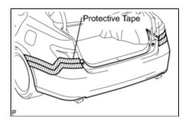
(a) Put protective tape around the rear bumper assembly.
