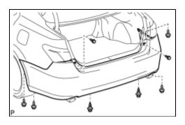
(c) Remove the 2 clips, 4 screws and 2 bolts.
