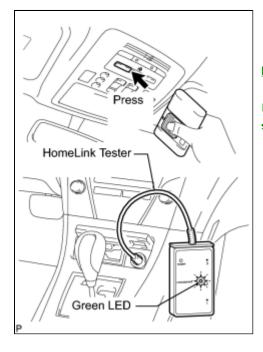
from the handheld transmitter. Check if the "HomeLink" tester's green LED illuminates.
