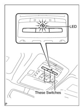
(a) To inspect the garage door opener system, press each switch and check that the LED in the "HomeLink" logo illuminates as illustrated. If one or more of the switches do not cause the LED to illuminate, confirm that the fuse and the wiring to the garage door opener system unit is normal. If the fuse and wiring are normal, and the LED does not work, replace the garage door opener system unit located in the roof console box assembly.
