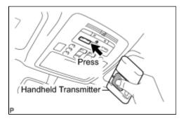
(a) Check if the tester's handheld transmitter code was successfully registered.
