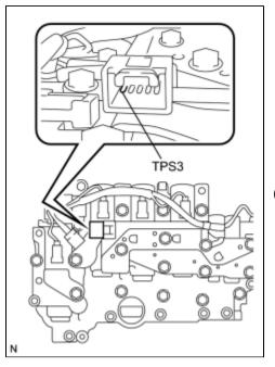
(a) Disconnect the connector from the ATF temperature sensor assembly.
